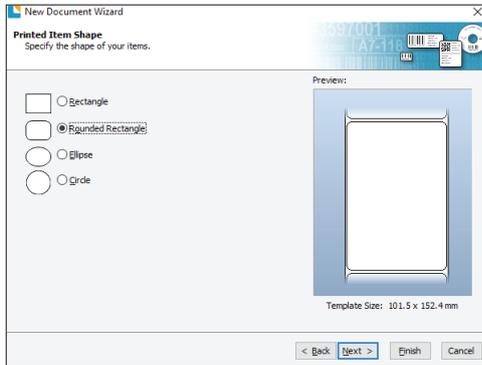
G. Insert your PDL size and in which direction you would like to print it. The size is the same as indicated on your Product Display Label Roll multiplying the length of the label by 2.
